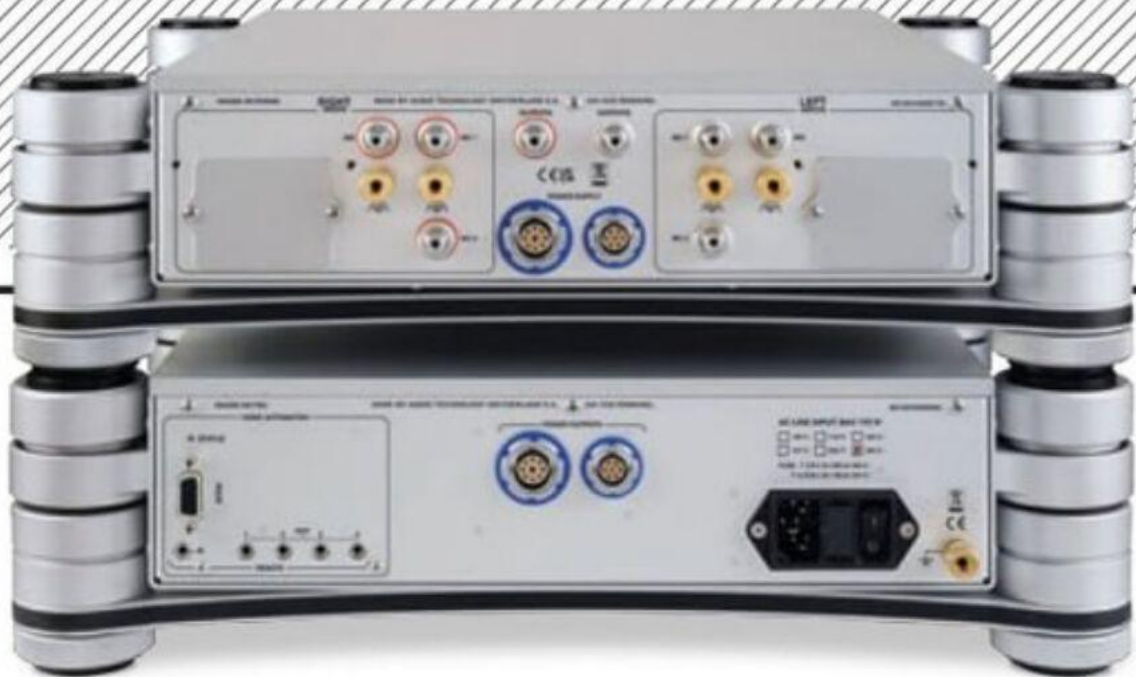
ABOVE: Phono preamp [top] has MM and 2x MC RCA inputs, each with an earth post, and RCA line outs. PSU [bottom] for the HD Phono's analogue (tube) circuits connects via a 9-pin LEMO socket [left], and for the digital (logic) via a 7-pin connector [right]
